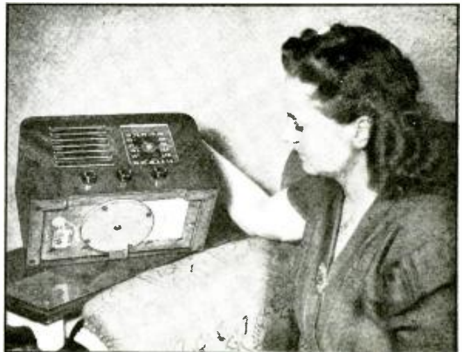
New "Roto Base" on RCA Little Nipper model 46X23 permits it to be turned in any direction, thus permitting the built-in loop antenna to be aimed directly at the wanted station thereby increasing signal strength.
